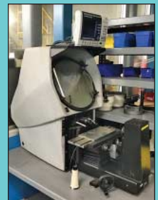
14" Scherr-Tumico Optical Comparator with Quadro-Chek 200, DRO
