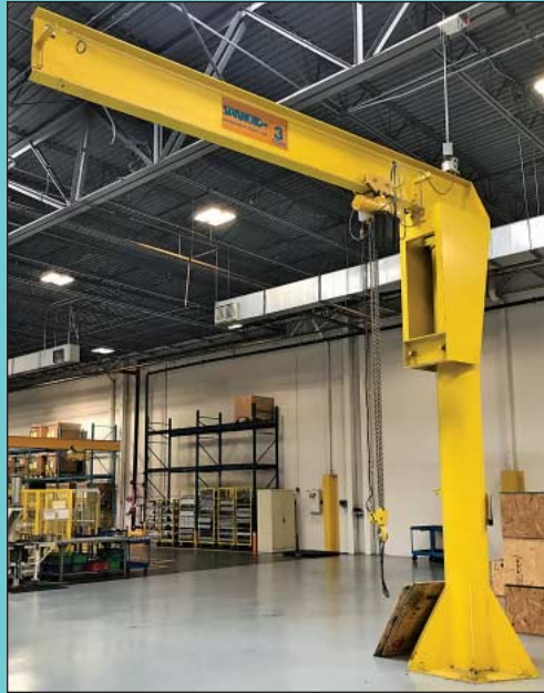
3 Ton X 16' Arm X 16' High Column Spanco Floor Mounted Jib Crane with 3 Ton Yale Chain Hoist
