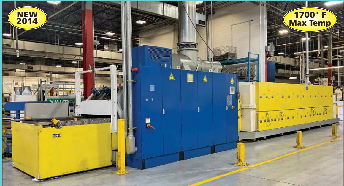
50" Wide Elinco Model FB-125/072/050-08EW.OC Electric Mesh Belt Conveyor Type Heat Treat Furnace
